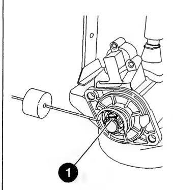
Checking clutch overrunning torque
